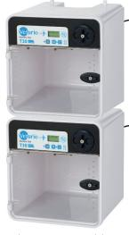
The Vetario 30 models can be stacked, the feet from one unit locate in sockets in the cabinet of the unit below.
